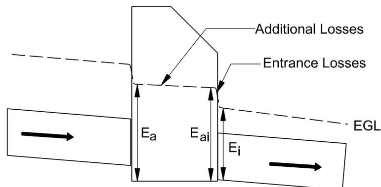
**Figure 12.13-C — DEFINITION SKETCH FOR HEC 22 (2009) MANHOLE LOSS METHOD**
