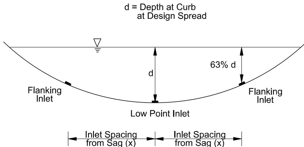
**Figure 12.10-D — FLANKING INLETS AT SAG POINT**
