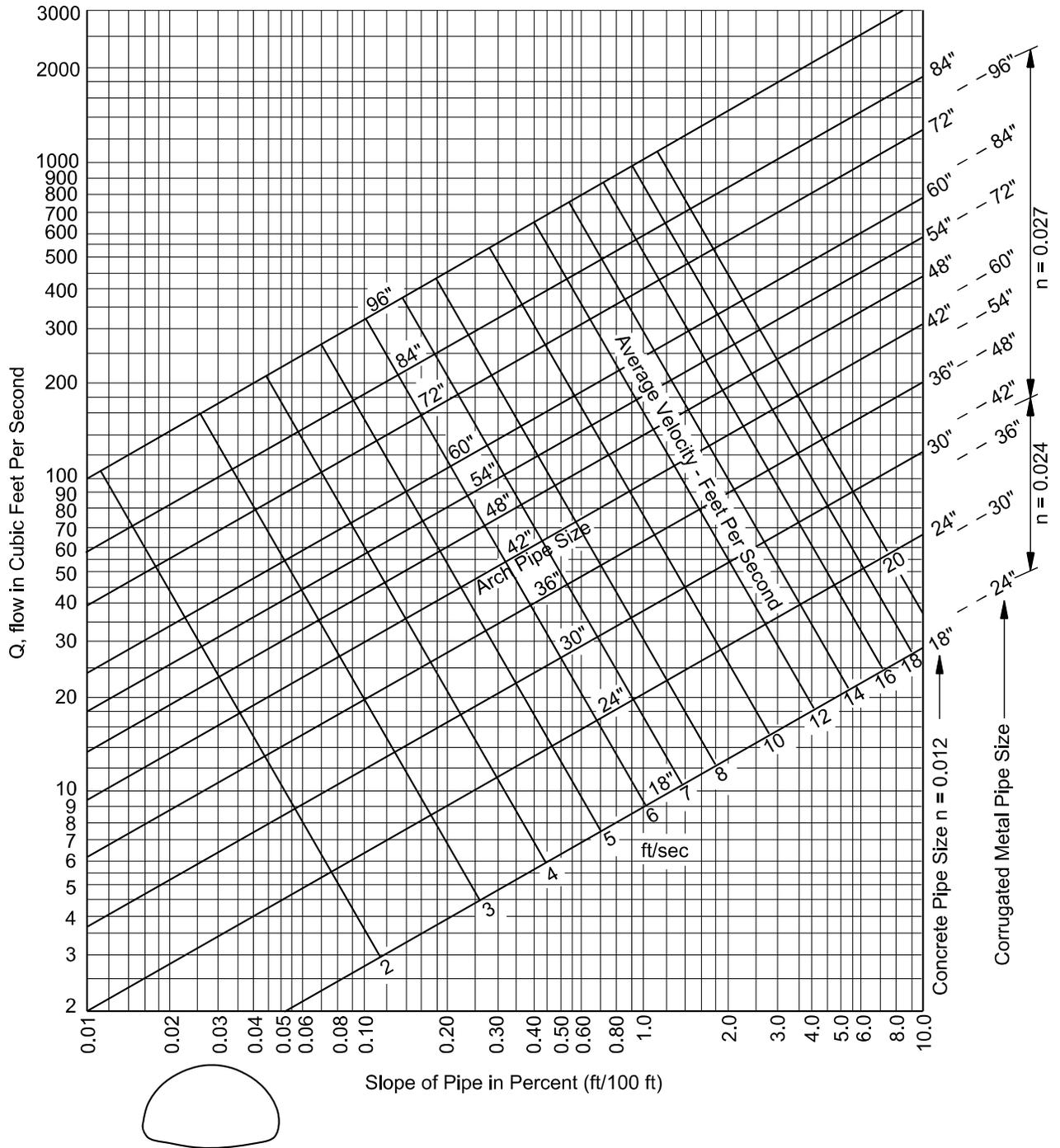
Figure 12.12-B — FULL-FLOW CURVES, ARCH PIPE,  $n = 0.012$
