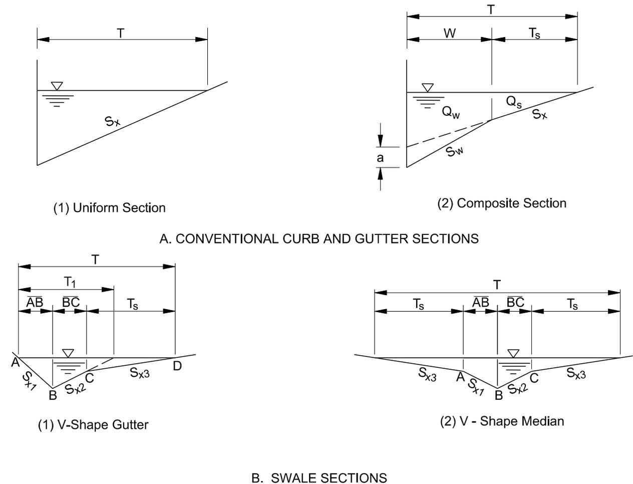
**Figure 12.8-A — TYPICAL CURB AND GUTTER SECTIONS**
