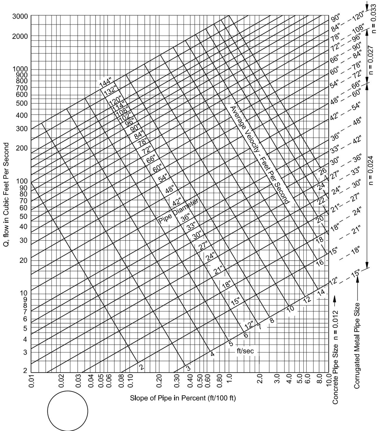
Figure 12.12-A — FULL-FLOW CURVES, CIRCULAR PIPE,  $n = 0.012$
