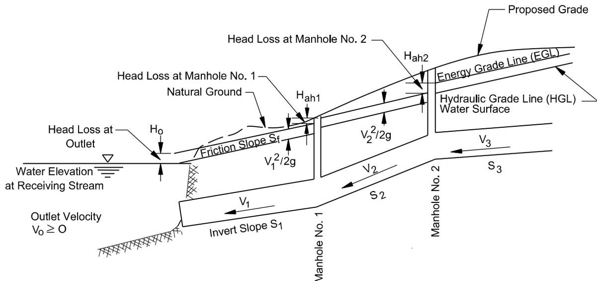
**Figure 12.13-A — HYDRAULIC AND ENERGY GRADE LINE ILLUSTRATION**
