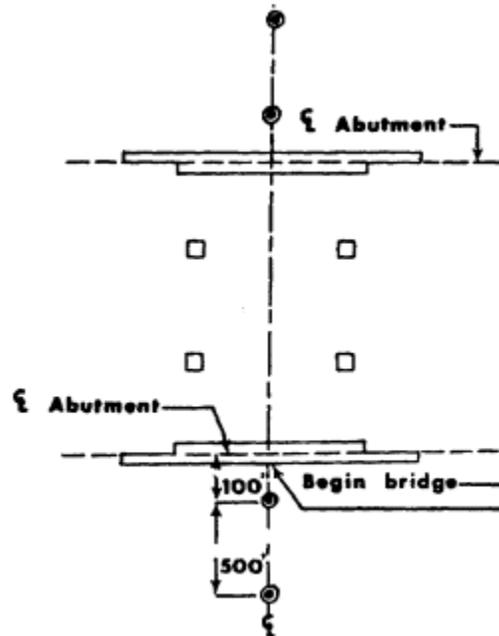
Set sufficient reference points to insure replacement, should one become damaged, or if it is known that a point will be disturbed, such as an approach fill.
