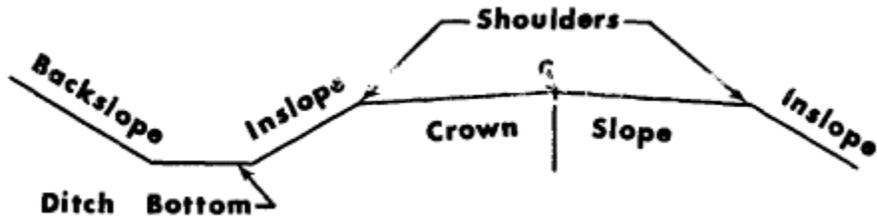
The angle of the inslope and backslope is given as a ratio, such as 4:1 or 3:1. The first number is the number of feet the slope must go horizontally to raise one foot vertically, the second number. (For metric numbers the ratio does not change; 3 meters horizontally vs. 1 meter vertically.)
