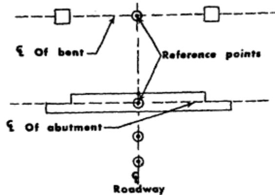
A minimum of two offset points should be set left and right of each bent or abutment reference point. These offset points should be set at right angles to the roadway centerline on straight bridges.
