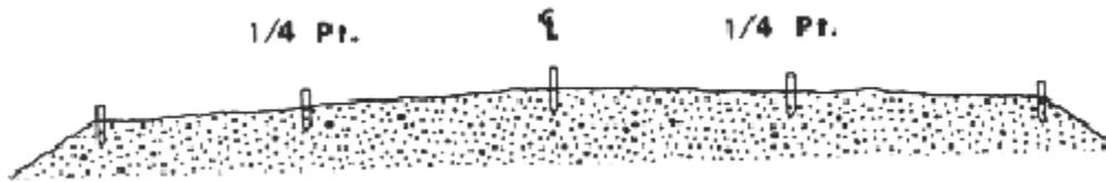
The edge of the driving lane is usually called the quarter point because it is about half way between the shoulder and centerline. These extra stakes make it easier for the equipment operators to finish the top of the roadway to the correct elevations. Without them there is a tendency to finish the roadway a little high or low at the quarter points.
