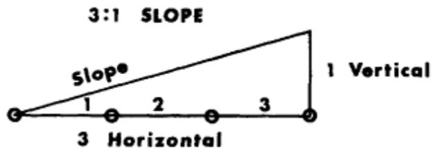
The crown slope is the rate that the road drops from the centerline to the shoulder. A typical crown slope rate is 0.02 feet per foot (2%). The purpose of this crown is to provide for water drainage.
