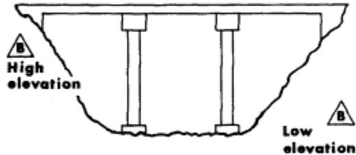
The new benchmarks established at a structure site should be checked from two different previously established benchmarks. This will reduce the possibility of error in the new benchmarks. Benchmarks need to be protected.
