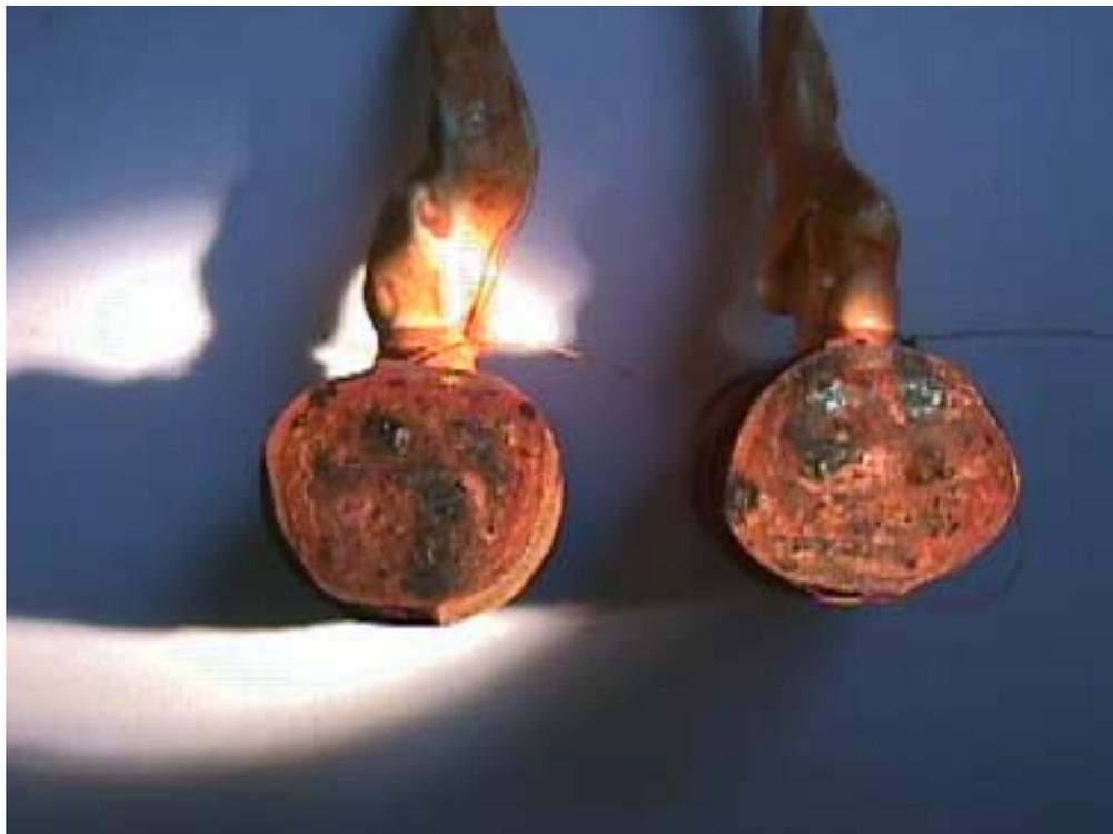
**Figure 18: Uncoated SSC Rebar After 8 Days at pH6, 60°C, Other Side Of Sample from Figure 17**
