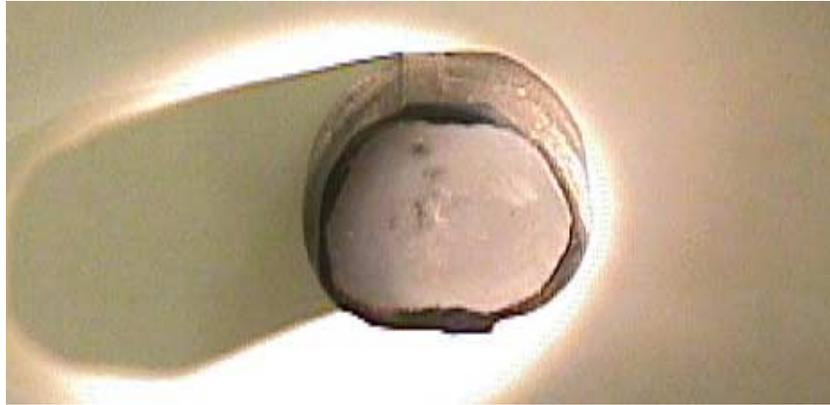
**Figure 7: Cut Surface a #6 SSC Bar**
