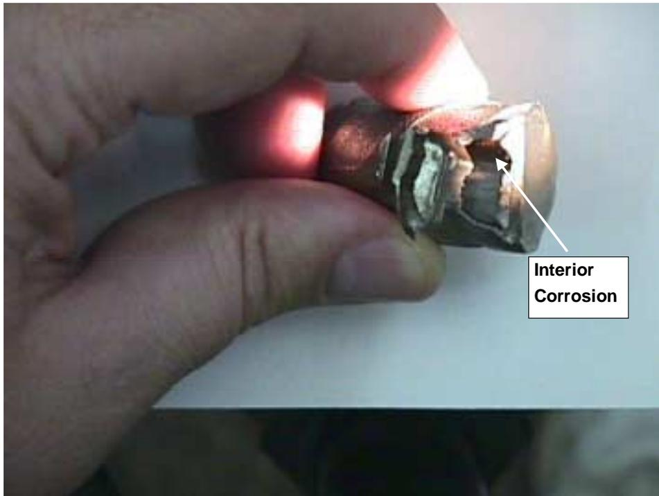
**Figure 2: Impact-Tested #6 SSC Rebar Showing Massive Internal Corrosion**
