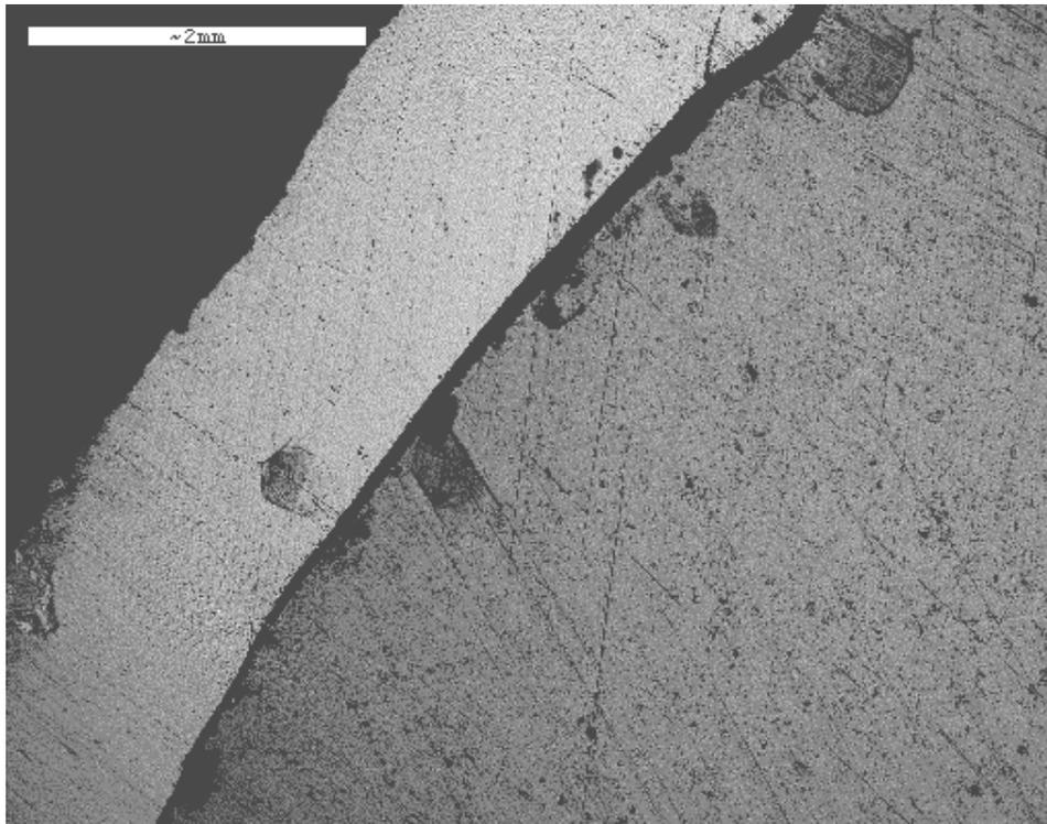
**Figure 3: Backscatter SEM Image of Core/Cladding Interface**
