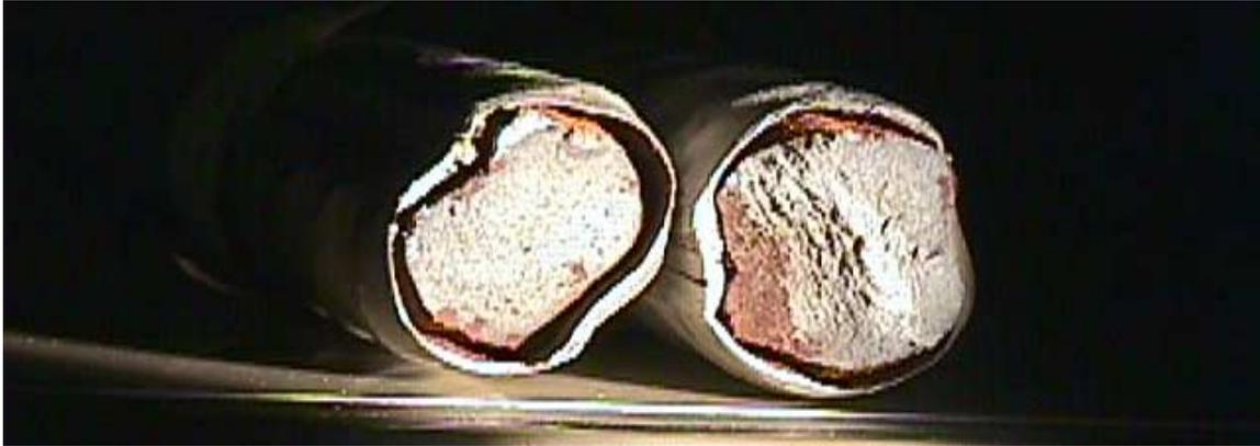
**Figure 5: Photograph of Tensile Test Failed SSC Rebar**
