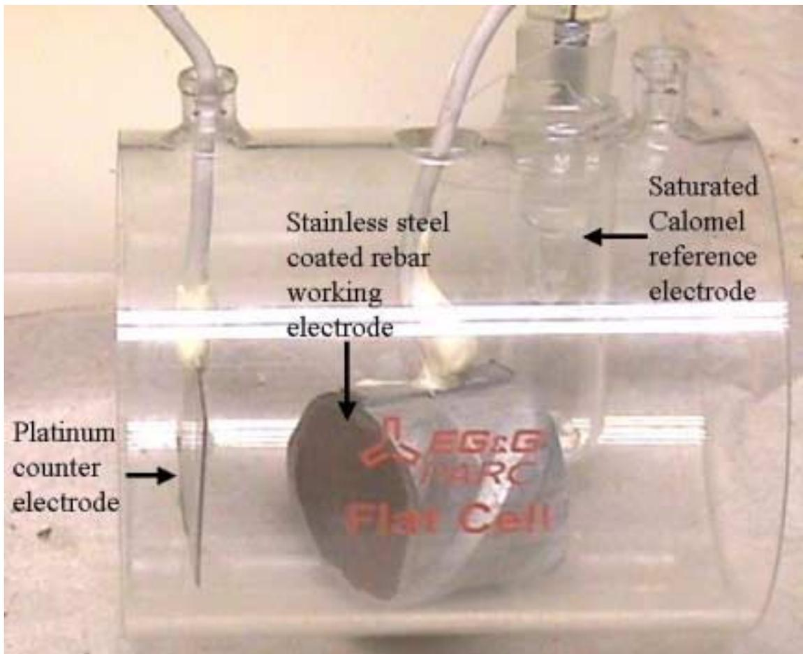
Figure 11: Electrochemical Cell with Electrodes in Place
