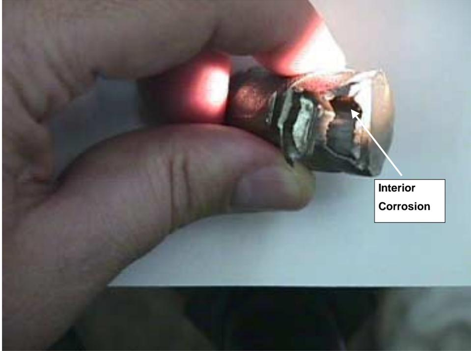
**Figure 20: Impact-Tested #6 SSC Rebar Showing Massive Internal Corrosion**
