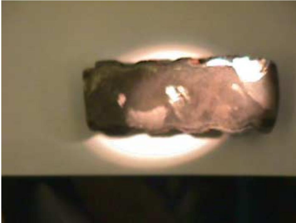
**Figure 19: Cross Section of Stainless Steel Coated SSC Rebar Tested 8 Days at pH6, 60°C**
