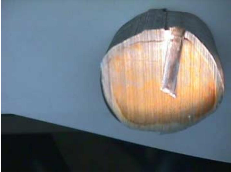
**Figure 21: #10 SSC Rebar After Impact Testing**
