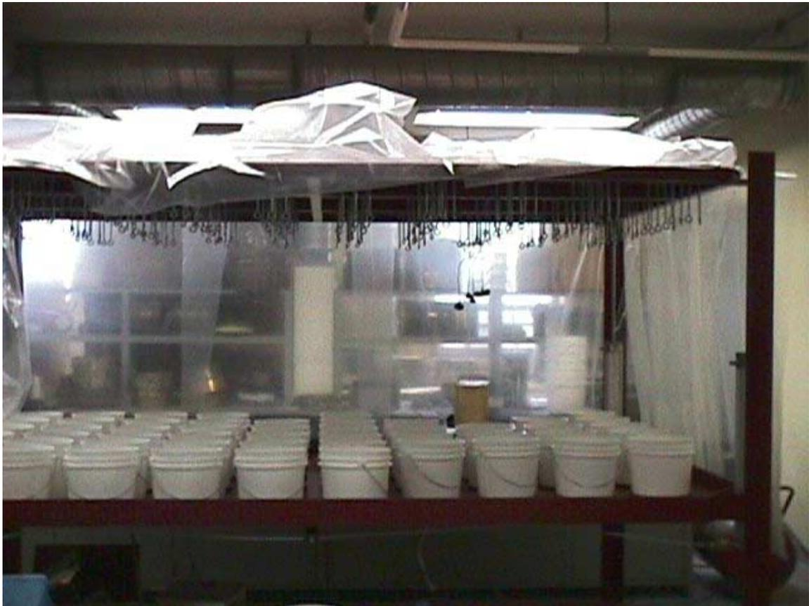
**Figure 12: Apparatus for Conducting Multiple Corrosion Tests Simultaneously**
