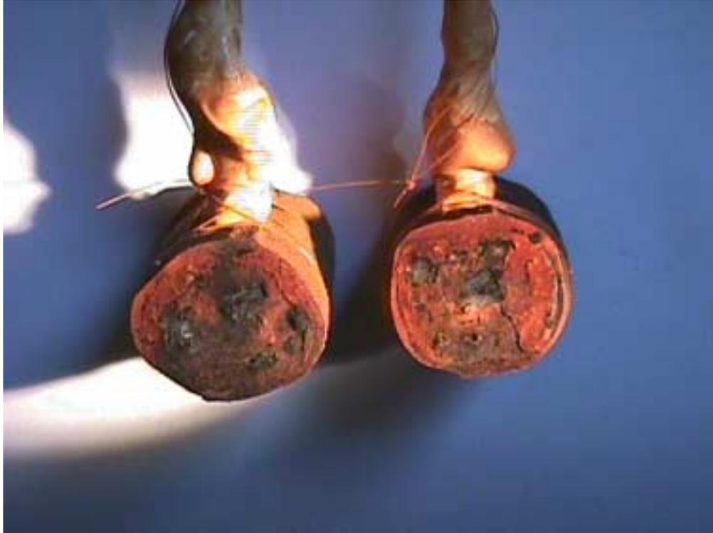
**Figure 17: Uncoated SSC Rebar After 8 Days at pH6, 60°C**
