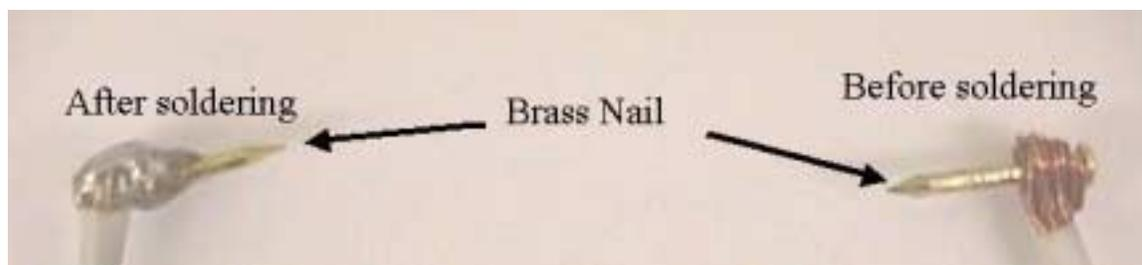
**Figure 9: Wire/Nail Assembly Before and After Soldering.**
