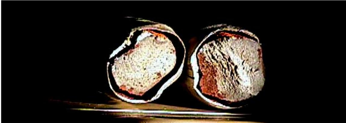
**Figure 1: Photograph of a tensile test failed SSC rebar**
